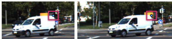
Figure 1. A car moving against a varying background. Nearly half of the patch centered on a Harris corner at the object boundary is part of the background.
