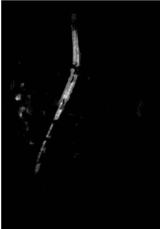
Figure 3.4: Figure where each individual pixel stores the number of times a foreground object was detected at that pixel. Note how the road is clearly distinguished from other areas due to objects moving on the road.
