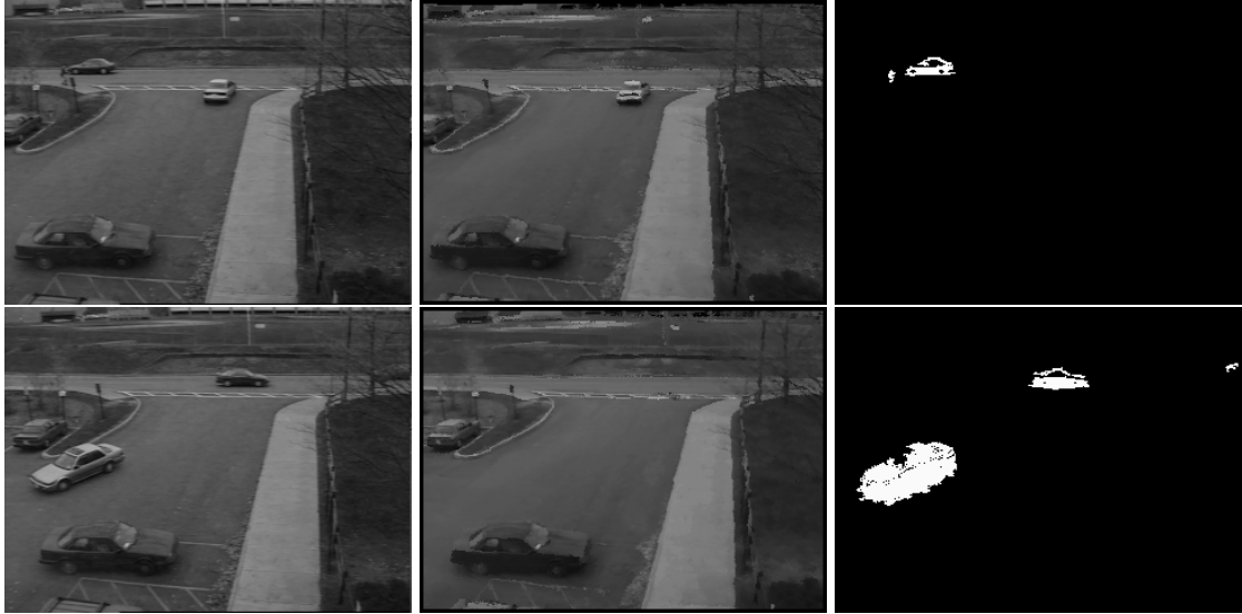
Figure 3.1: (a) Two views of a parking lot using a moving surveillance camera, (b) synthesized frames with foreground objects removed, and (c) the moving objects detected. Note that very small objects, such as a person walking and a car entering behind trees were correctly detected.
