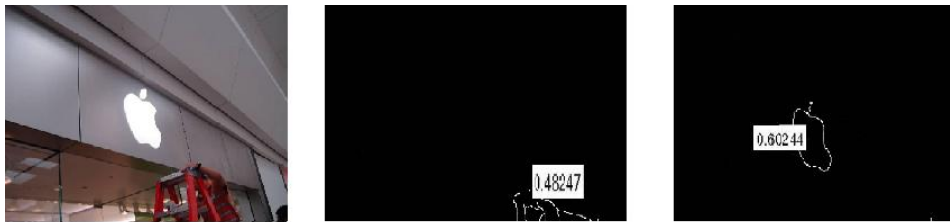
Figure 11: (top) A test image. (bottom) Two traced contour groups for the object bounding boxes detected at the first stage. The first detection was discarded while the second was taken as a true detection by the Verification stage.
