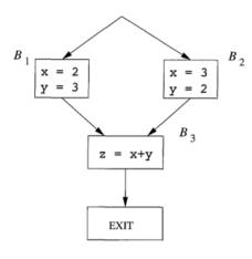
Say  $f_1$ ,  $f_2$ , and  $f_3$  represent the transfer functions of  $B_1$ ,  $B_2$  and  $B_3$ , respectively.  $f_3(f_1(m_0) \land f_2(m_0)) \sqsubseteq$  $f_3(f_1(m_0)) \land f_3(f_2(m_0))$
