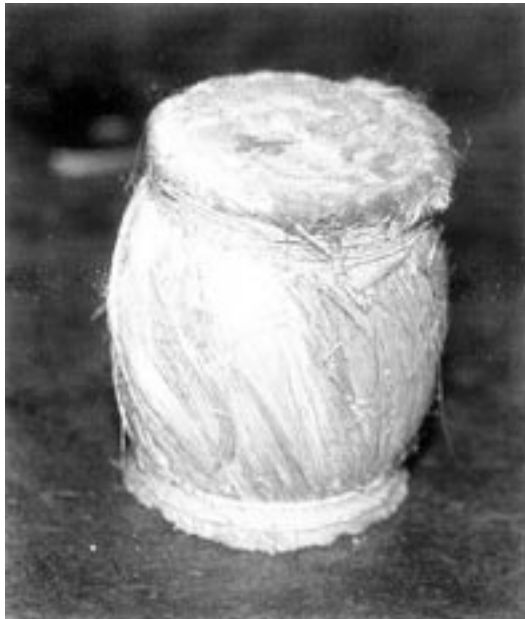
Fig. 12. One of the twisted-jute polarizers used by Bose.
