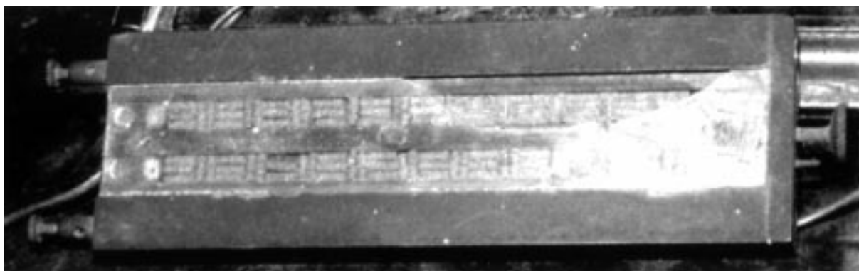
Fig. 8. One of Bose's free-space radiation receivers, recently described [3] as a "space-irradiated multi-contact semiconductor (using the natural oxide of the springs)." The springs are kept in place in their tray by a sheet of glass, seen to be partly broken in this photograph.
