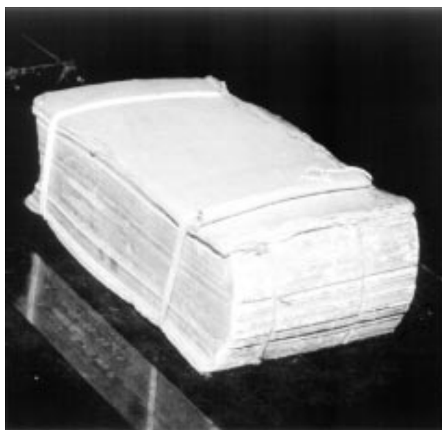
Fig. 10. One of Bose's polarizers was a cutoff metal-plate grating, consisting of a book (Bradshaw's Railway Timetable ) with sheets of tinfoil interleaved within the pages.
