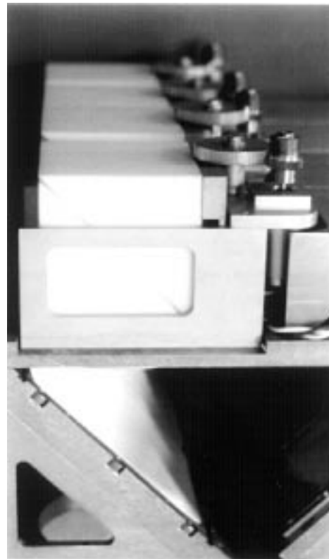
Fig. 15. Four of the eight double-prism attenuators used to control local-oscillator injection into the NRAO 1.3-mm eight-beam receiver in use on the 12-m telescope at Kitt Peak.
