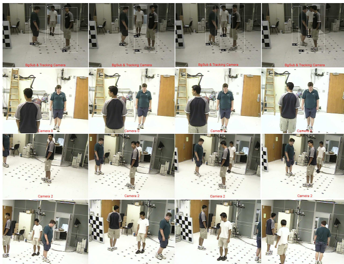
Fig. 13 Row 1: The three persons first appeared sufficiently separated to be detected individually (left image, row 1). Given only two active cameras, person 0 and 2 was scheduled first. Because the system was able to track through occlusions, shown in row 1, so that the image of person 0 was prevented from merging with those of person 1 and 2 as they were captured, the predicted motion model of person 0 was accurate enough for camera 2 to capture unobstructed and well-magnified frames of person 0 after it finished capturing person 2, shown in row 4. Row 2: Capturing person 1 with camera 0. Row 3: Capturing person 2 with camera 2. Row 4: Capturing person 0 with camera 2 after person 2.
