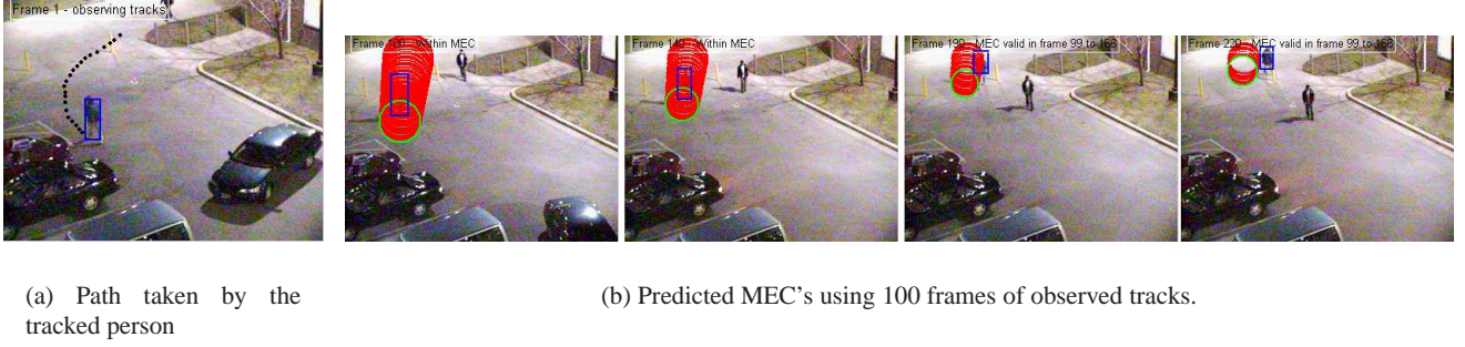
Fig. 4 In (b), red circles represent the MEC's predicted for the following frames, while the green circle represents the predicted location in the current frame. Comparing these circles with the positions given by the tracker (blue bounding box), the prediction were sufficiently accurate, as shown in (b), for the required number of frames, even though the person was walking along a curved path as shown in (a).
