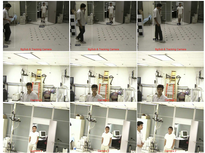
Fig. 10 Row 1: The motion models of two people in the scene were used to determine when they are front-facing to the assigned camera (two active cameras are used here), for face capture. This is illustrated in rows 2 and 3, where each person is front-facing to only one of the movable cameras, which was then assigned to the task accordingly. Here, the right image shows the scheduler annotating the bounding boxes with the ID of the assigned camera. The TVI of person 0 in this example is delimited by the predicted crossing with person 1. Row 2: Frames showing camera 0 capturing person 1's face. Row 3: Frames showing camera 2 capturing person 0's face.
