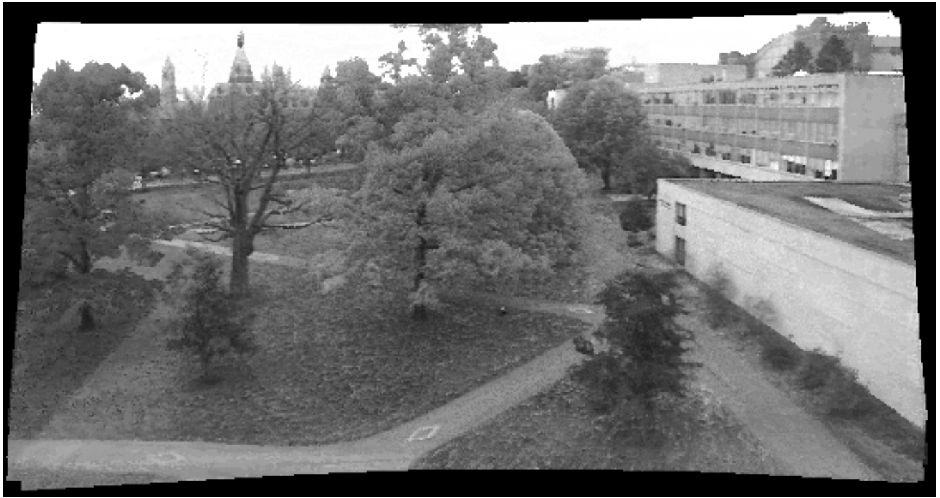
Figure 6: The background mosaic from a sequence of 1000 frames captured from a surveillance camera moving in both vertical and horizontal directions
