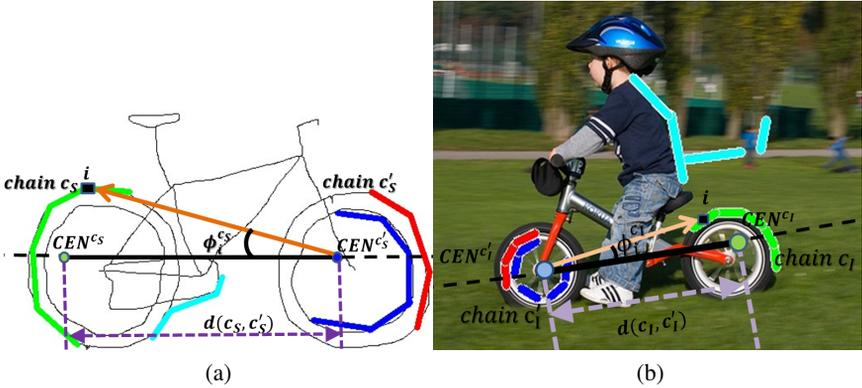
Fig. 4: Pairwise geometric consistency of the matched portions of a chain pair  $\mathbf{p} = (C_S, C_I)$  with respect to  $\mathbf{p}' = (C'_S, C'_I)$  uses (i) the distances  $d(C_S, C'_S)$  and  $d(C_I, C'_I)$  between their centroids (CEN) and (ii) the difference of angles  $|\phi_i^{C_S} - \phi_i^{C_I}|$ .
