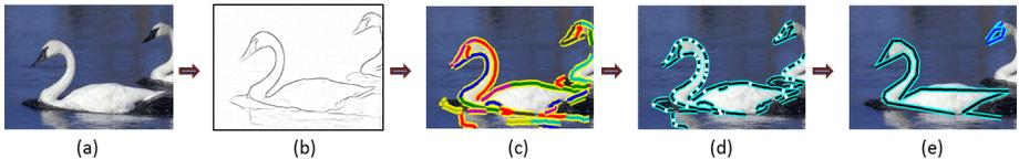
Fig. 1: Creation of chains: (a) Original image, (b) Berkeley edge-map [1], (c) Salient contours [45] extracted, (d) Extracted straight line-like segments, (e) Final chains obtained (black and blue).
