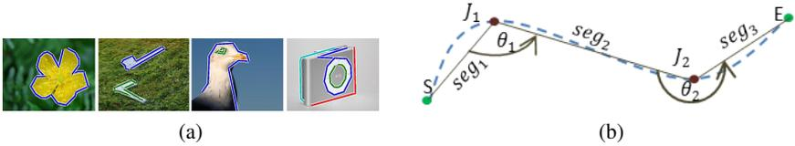
Fig. 2: Image Representation: (a) Chains extracted for some images. Different chains are represented using different colors. (b) The chain for the curve SE is composed of three line segments. The descriptor for this chain is  $\Psi = \langle \gamma_i = \frac{l_{seg_i}}{l_{seg_{i+1}}}, \theta_i \mid i \in \{1, 2\} \rangle$ .
