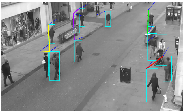
Figure 2. MSTs of clusters (groups) after clustering on a sample frame from Oxford Town Center dataset [3]. The bounding boxes are connected with colored lines that represents the tree and the blue lines show the direction of pedestrians.
