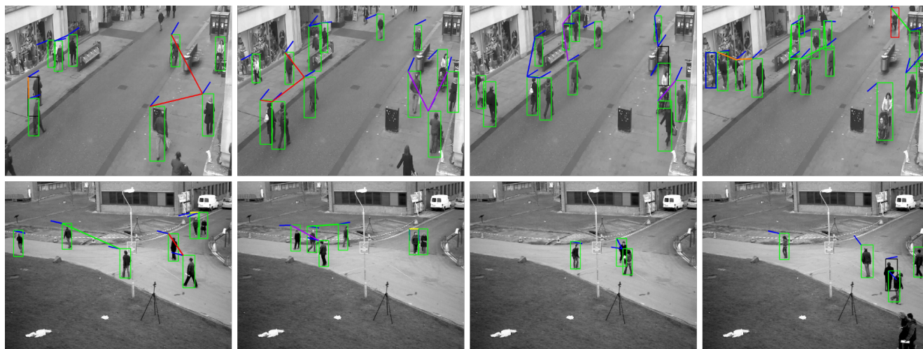
Figure 5. Sample results from Oxford Town Center dataset [3] in first row, and from PETS 2009 L1 dataset in second row. The green rectangles show pedestrians being tracked, the red show leaving pedestrians, the black show occluded, and the blue show newly entered pedestrians.
