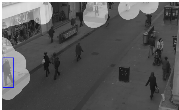
Figure 4. Bright regions contain possible new pedestrians which are not being tracked. A newly entered pedestrian is shown with blue bounding box.
