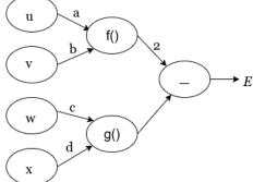
Here u, v, w, x are inputs (constants) and a, b, c, d are parameters (variables). f and g are the activation functions (with z as input) defined as below:
