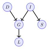
•  $(G \not\perp D)$   $(G \not\perp I)$   $(S \not\perp I)$   $(L \not\perp G)$ A node is not independent of its parents
