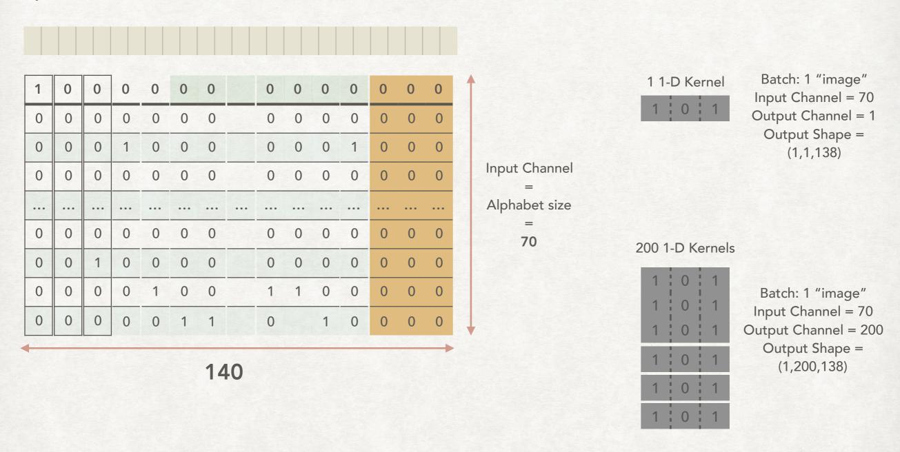
Max pooling operation will result in a 200 dimensional embedding for each "image" Note that this kernel covers tri-gram, there could be other which can cover bi-gram, five-grams etc.
