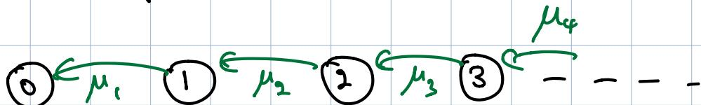
$$Q = \begin{bmatrix} 0 & 1 & 2 & \cdots \\ 0 & \mu_1 & -\mu_1 & & \\ 1 & \mu_2 & -\mu_2 & \ddots & \\ 2 & & & \ddots & \\ \vdots & & & \ddots & \\ \vdots & & & \ddots & \end{bmatrix}$$
