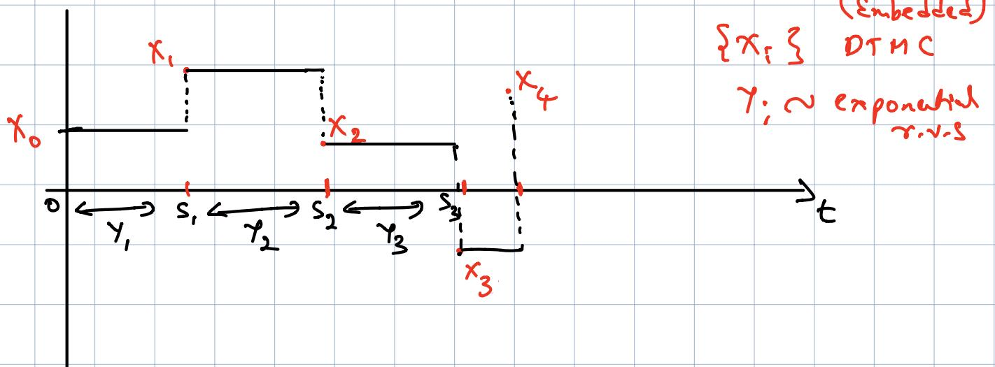
Spl. case:  $X_i = X_{i-1} + 1$  &  $Y_i \sim \text{Exp}(\lambda)$  lead to Poisson process with rate  $\lambda$ .
