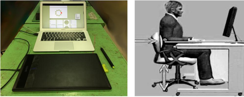
Fig. 4.1: Experimental setup for the 2D Fitts's Law based experiment. The left side figure is the apparatus used for conducting the experiment. It consists of a Wacom™ Graphics tablet which is connected to a system. The right side figure is from Raghu Prasad *et al.* (2013) and is the standard sitting posture that is maintained for the experiment. It ensures proper comfort during the experiment.
