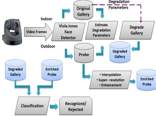
Fig. 3. The proposed framework for compensating degradation, for Face Recognition from a surveillance video.
