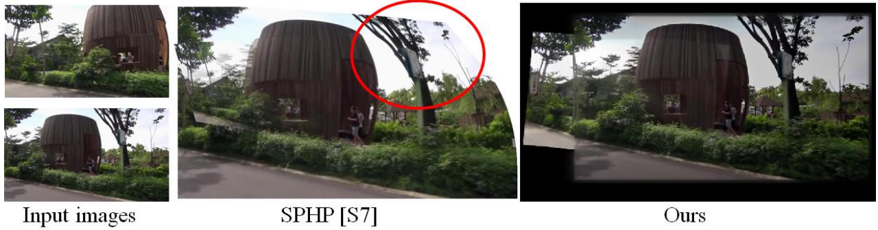
Fig. S32: Qualitative comparison of performance with the method SPHP [S7], for a pair of frames taken from an unconstrained video, Parallax2 , of our dataset (Section A). SPHP produces distortions towards the right top end of the stitched image as seen in the region marked in red oval boundary, whereas our method produces the desired output.
