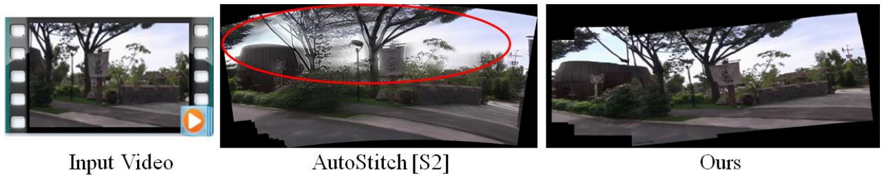
Fig. S12: Qualitative Comparison for panorama generation of our method with AutoStitch [S2] for Parallax2 . AutoStitch causes ghosting artifacts throughout the stitched image. The red oval boundary highlight the ghosting effects.
