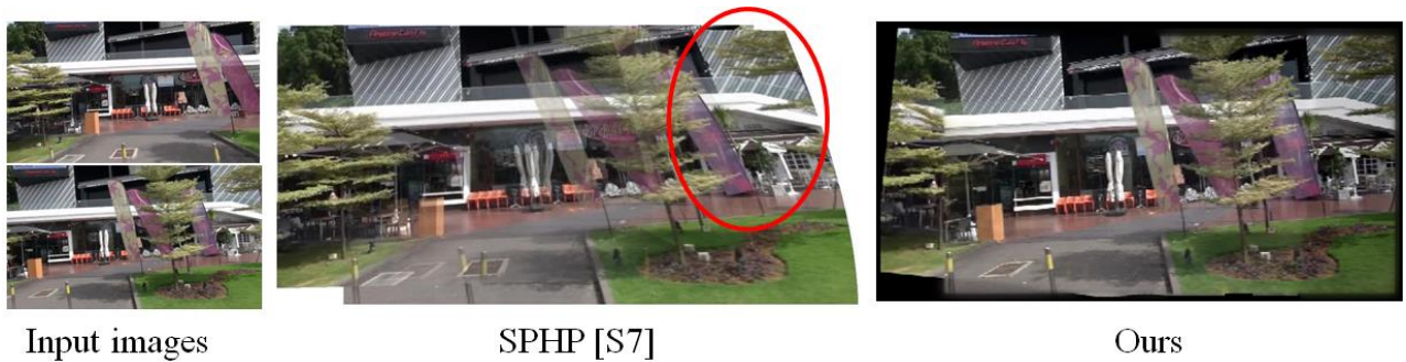
Fig. S33: Qualitative comparison of performance with the method SPHP [S7], for a pair of frames taken from an unconstrained video, Run2 , of our dataset (Section A). SPHP produces distortions towards the right top end of the stitched image as seen in the region marked in red oval shape, whereas our method produces the desired output.
