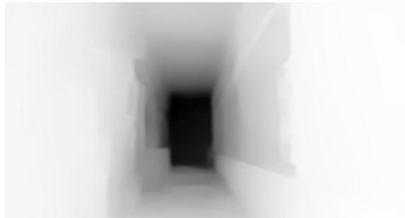
A grayscale depth map of the hallway, showing a dark central area representing the floor and lighter areas representing the walls and ceiling.                   |
