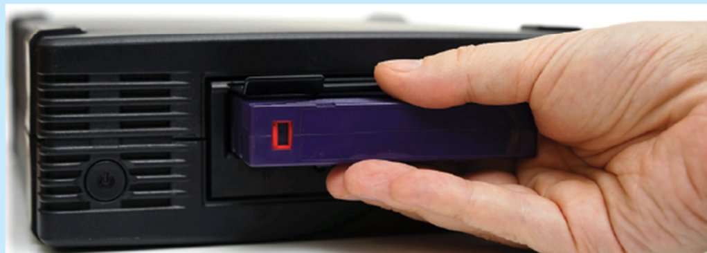
Figure 11.5 An LTO-6 Tape drive with tape cartridge inserted.
