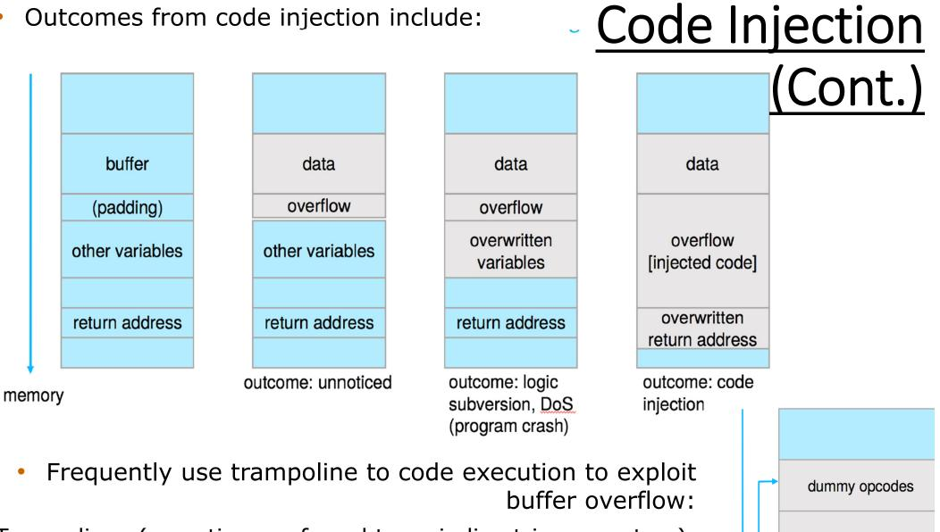
Trampolines (sometimes referred to as indirect jump vectors) are memory locations holding addresses pointing to interrupt service routines, I/O routines, etc. Execution jumps into the trampoline and then immediately jumps out, or bounces, hence the term trampoline.
