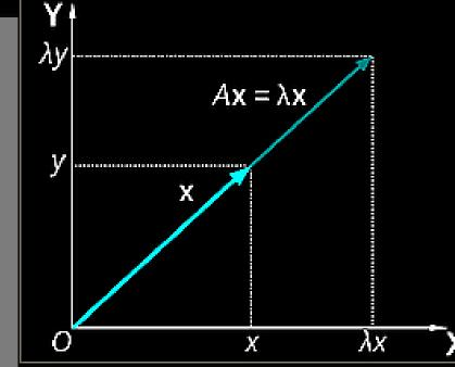
Matrix A acts by stretching the vector  $\mathbf{x}$ , not changing its direction, so  $\mathbf{x}$  is an eigenvector of A.
