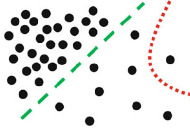
Fig. 6.20 Illustrating the strong bias of non-normalized graph cuts in the absence of terminal nodes. The green dashed line indicates a suitable cut of the point set, whereas non-normalized cuts rather produce cuts indicated by the dotted red curve
