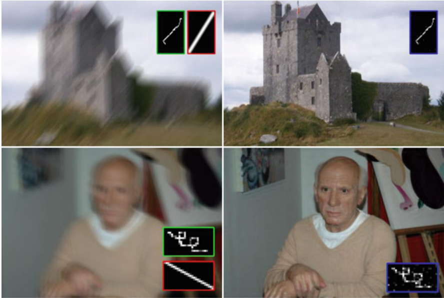
Fig. 4.9 Illustrating the performance of the blind deconvolution algorithm proposed in [23]. The left column depicts the blurred image. The reconstructed image is depicted in the right column . All examples are shown together with the true kernel ( box framed green ), the initial kernel estimate ( box framed red ), and the final kernel estimate ( box framed blue ) (Shan et al. [23] © 2008 Association for Computing Machinery, Inc. Reprinted by permission)
