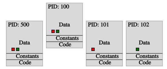
We can arrange for each forked (child) process to have access to only one shared memory block. The parent can access all shared memory blocks.
