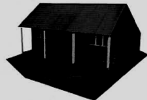
Fig. 10.5. Metric reconstruction. The affine reconstruction of figure 10.4 is upgraded to metric by computing the image of the absolute conic. The information used is the orthogonality of the directions of the edges of the building.
