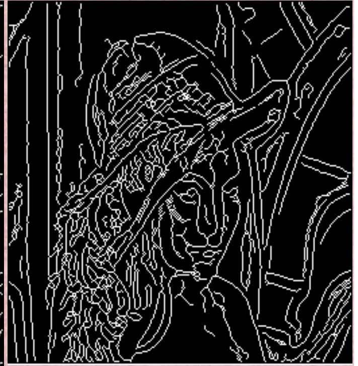
Edge map generated by scale space Combination
