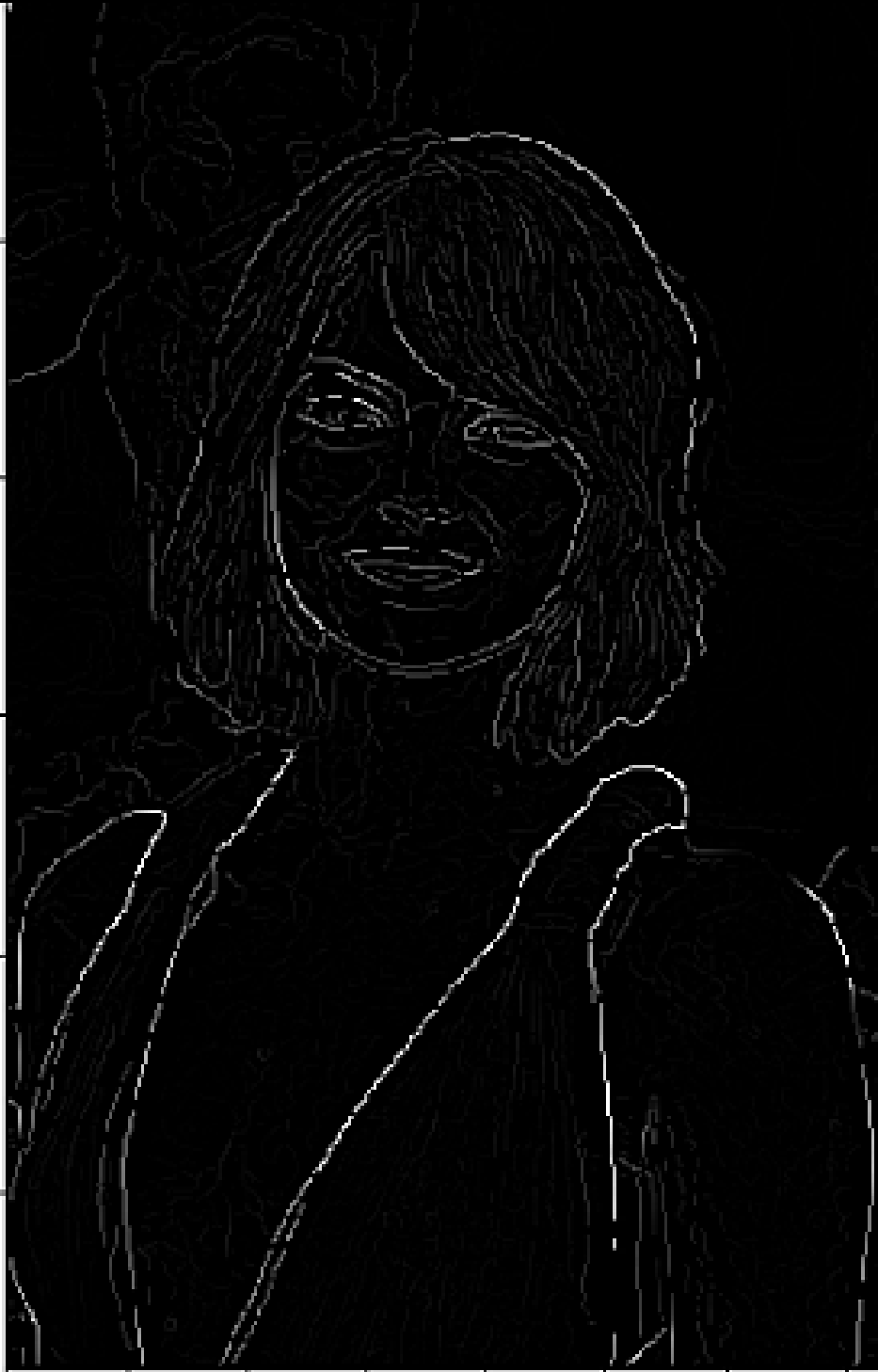
Non-Max Suppression image (left) — Bi-level Thresholding result (right): weak pixels in gray and strong ones in white.
