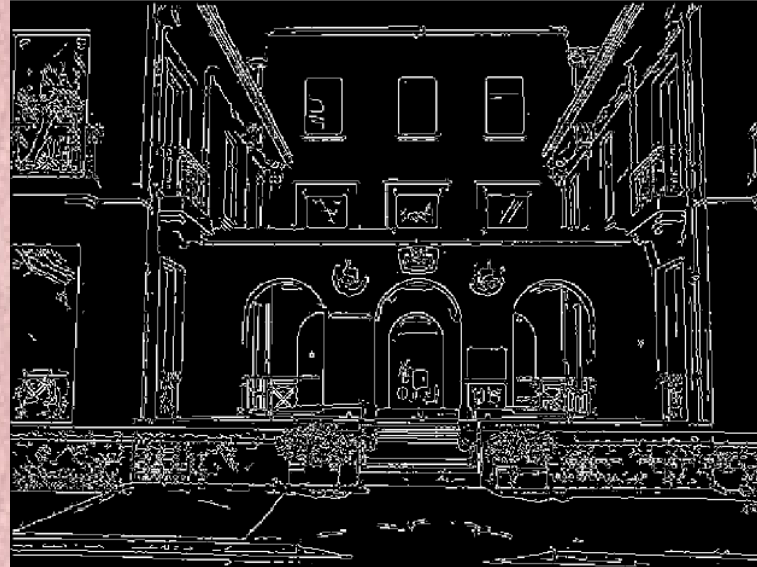
Strong + connected weak edges
