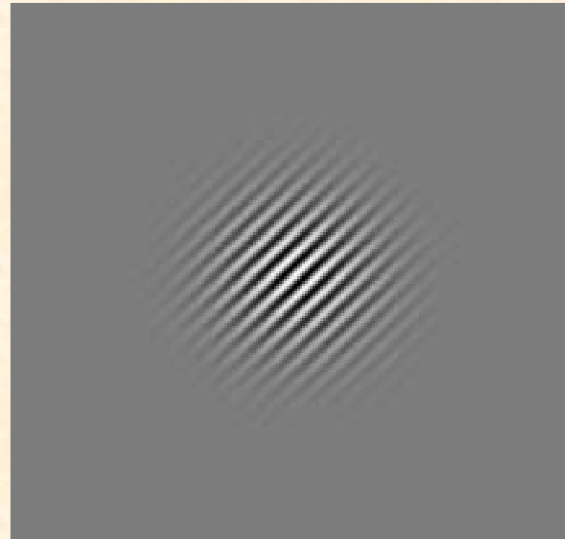
A typical Gabor filter with \sigma=30 , \omega=3.14 and \theta=45^\circ
