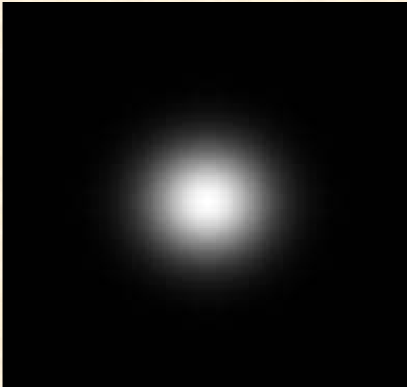
A typical Gaussian filter with \sigma=30
