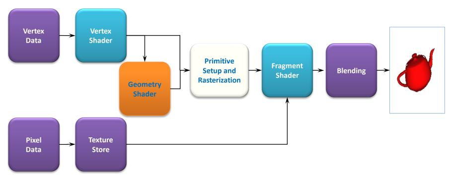
OpenGL version 3.2 added a new shader stage called *geometry shading* which allows the modification (and generation) of geometry within the OpenGL pipeline.
