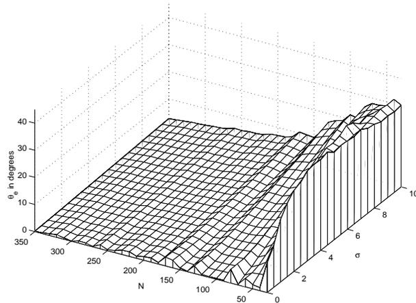
**Figure 6.** 3-D Plot showing the errors in reconstruction,  $N$  varies from  $[30 - 350]$ ,  $l = m = n = \frac{1}{\sqrt{(3)}}$ ,  $\sigma$  varies from  $[0 - 10]$ ,  $\alpha_1 = \beta_2 = \frac{2\pi}{3}$ ,  $\gamma_3 = \frac{\pi}{6}$ ,  $f_1 = f_2 = 1.0$ ,  $x_d = 10.0$ ,  $y_d = 20.0$ ,  $z_d = 30.0$ ,  $x_w = y_w = 10.0$  and  $z_w = 200.0$ .
