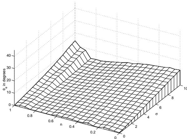
**Figure 5.** 3-D Plot showing the errors in reconstruction,  $n$  varies from  $[0 - 1]$ ,  $l = m = \sqrt{\frac{(1-n^2)}{2}}$ ,  $\sigma$  varies from  $[0 - 10]$ ,  $\alpha_1 = \beta_2 = \frac{2\pi}{3}$ ,  $\gamma_3 = \frac{\pi}{6}$ ,  $f_1 = f_2 = 1.0$ ,  $x_d = 10.0$ ,  $y_d = 20.0$ ,  $z_d = 30.0$ ,  $x_w = y_w = 10.0$ ,  $z_w = 200.0$  and  $N = 320$ .
