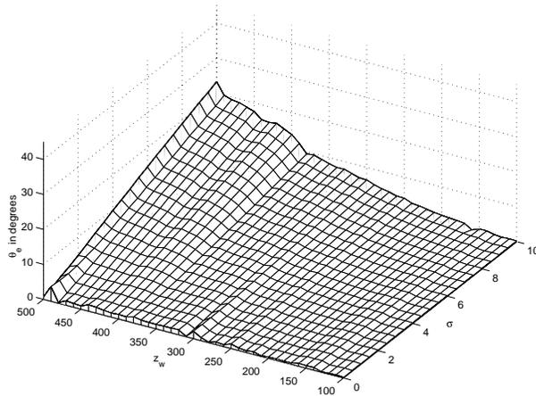
**Figure 7.** 3-D Plot showing the errors in reconstruction,  $z_w$  varies from  $[100 - 500]$ ,  $l = m = n = \frac{1}{\sqrt{3}}$ ,  $\sigma$  varies from  $[0 - 10]$ ,  $\alpha_1 = \beta_2 = \frac{2\pi}{3}$ ,  $\gamma_3 = \frac{\pi}{6}$ ,  $f_1 = f_2 = 1.0$ ,  $x_d = 10.0$ ,  $y_d = 20.0$ ,  $z_d = 30.0$ ,  $x_w = y_w = 10.0$  and  $N = 640$ .
