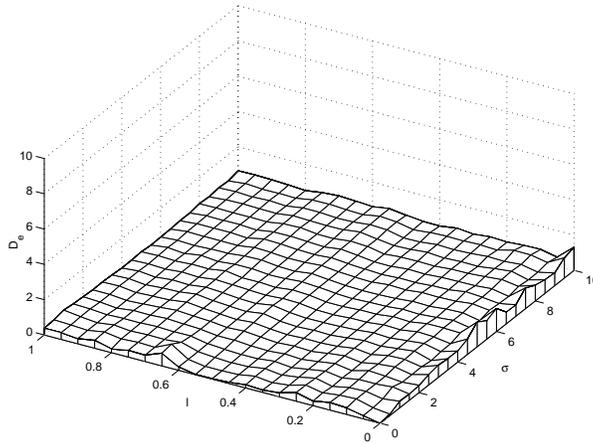
**Figure 9.** 3-D Plot showing the errors in reconstruction,  $l$  varies from  $[0 - 1]$ ,  $m = n = \sqrt{\frac{(1-l^2)}{2}}$ ,  $\sigma$  varies from  $[0 - 10]$ ,  $\alpha_1 = \beta_2 = \frac{2\pi}{3}$ ,  $\gamma_3 = \frac{\pi}{6}$ ,  $f_1 = f_2 = 1.0$ ,  $x_d = 10.0$ ,  $y_d = 20.0$ ,  $z_d = 30.0$ ,  $x_w = y_w = 10.0$ ,  $z_w = 200.0$  and  $N = 320$ .
