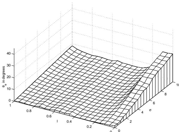
**Figure 3.** 3-D Plot showing the errors in reconstruction,  $l$  varies from  $[0 - 1]$ ,  $m = n = \sqrt{\frac{(1-l^2)}{2}}$ ,  $\sigma$  varies from  $[0 - 10]$ ,  $\alpha_1 = \beta_2 = \frac{2\pi}{3}$ ,  $\gamma_3 = \frac{\pi}{6}$ ,  $f_1 = f_2 = 1.0$ ,  $x_d = 10.0$ ,  $y_d = 20.0$ ,  $z_d = 30.0$ ,  $x_w = y_w = 10.0$ ,  $z_w = 200.0$  and  $N = 320$ .
