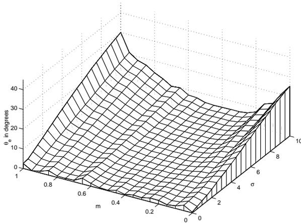
**Figure 4.** 3-D Plot showing the errors in reconstruction,  $m$  varies from  $[0 - 1]$ ,  $l = n = \sqrt{\frac{(1-m^2)}{2}}$ ,  $\sigma$  varies from  $[0 - 10]$ ,  $\alpha_1 = \beta_2 = \frac{2\pi}{3}$ ,  $\gamma_3 = \frac{\pi}{6}$ ,  $f_1 = f_2 = 1.0$ ,  $x_d = 10.0$ ,  $y_d = 20.0$ ,  $z_d = 30.0$ ,  $x_w = y_w = 10.0$ ,  $z_w = 200.0$  and  $N = 320$ .
